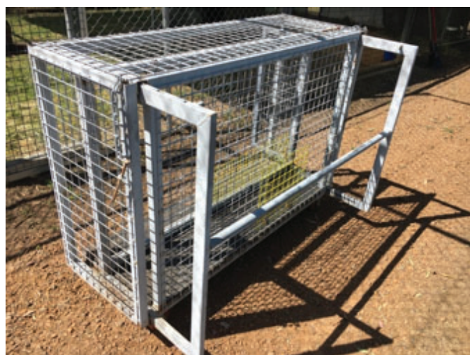
Image 1: The original chute design with sliding wall and wheels
